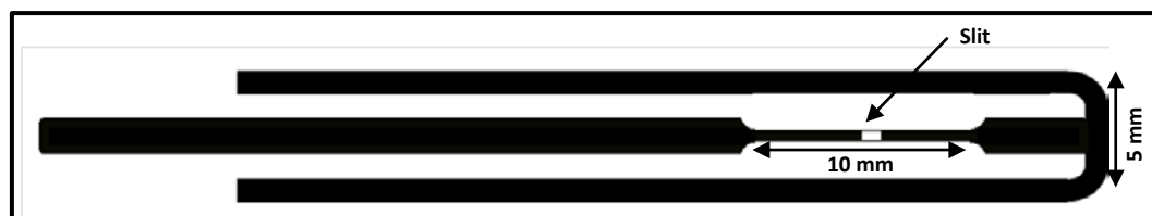
Figure 2.22 Optical mask to fabricate the slotted microcoils using photolithography
