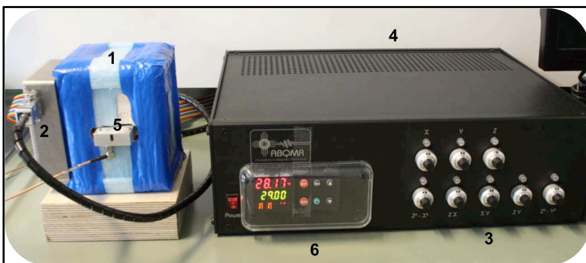
Figure 2.19 Portable NMR instrument: 1) 1.6 T permanent magnet, 2) control for heater pads and shims, 3) shim control electronics, 4) radio processor, 5) tuning/matching circuit box with microprobe, and 6) temperature control unit
