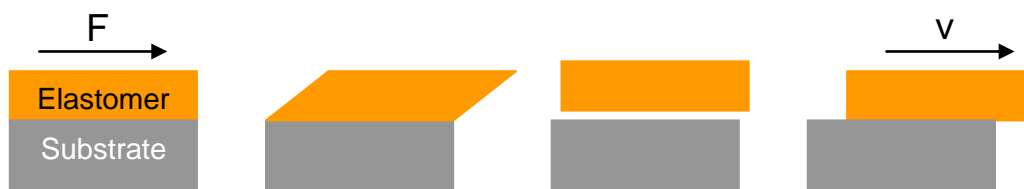
Figure 129: Schematic diagram of a stick-slip cycle – sticking, deformation, detachment, re-contact
