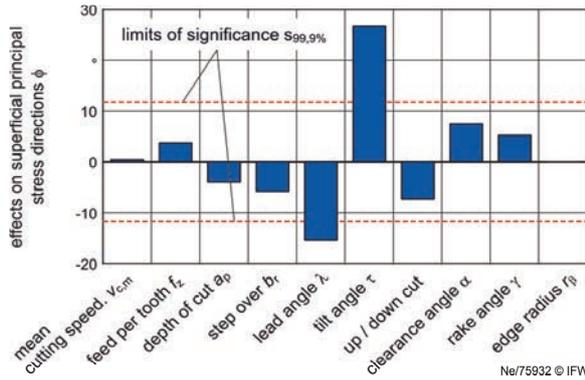
Fig. 2. Result of the fractional factorial design
