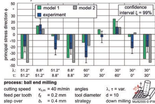
Fig. 6. Comparison of measured and predicted principal stress direction
