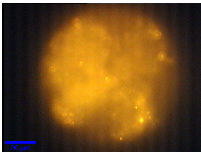
Figure 0.1: Surface of an anaerob ammonium oxidizing (ANAMMOX) biofilm granule. Light microscopic image taken with the CRM 200 (white light illumination; Nikon CFI Fluor water-immersion objective).
