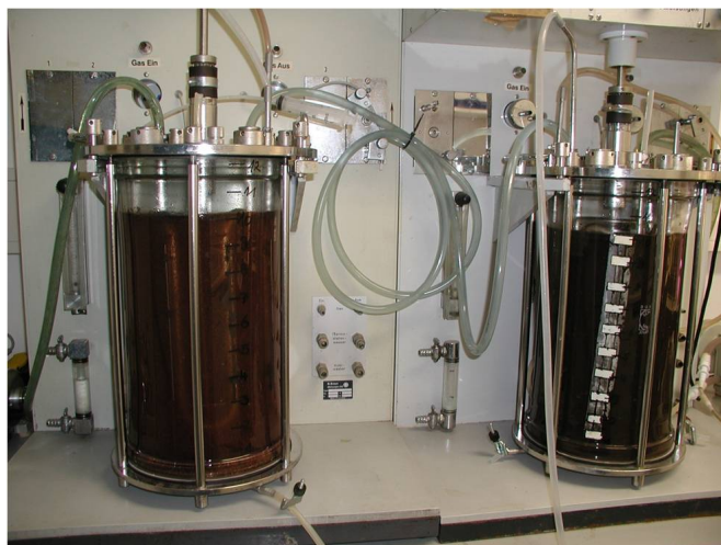
Figure 2.4: Sequencing batch reactors (SBR) for anaerobic ammonium oxidization at the Institute of Biophysics. Photo kindly provided by Dr. I. Wesoly.
