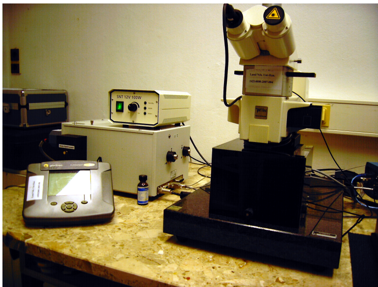
Figure 2.1: Confocal Raman microscopy workstation with the CRM 200 and SDU-1 at the institute of biophysics.
