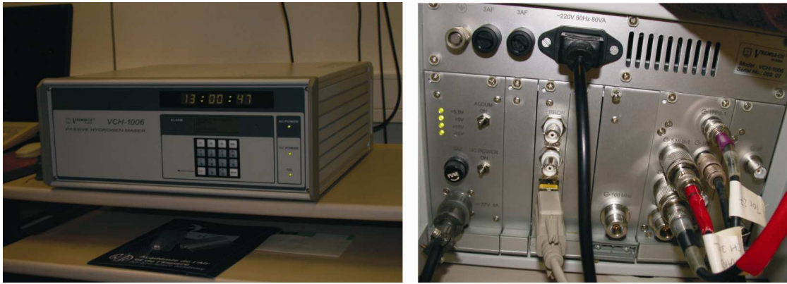
Figure 3.2.: Maser VCH-1006: The left photo shows the front view, the right photo points out the multiplicity of 1 PPS and frequency outputs. The signals can be distributed to the GPS receiver and a measuring system without additional amplifiers.
