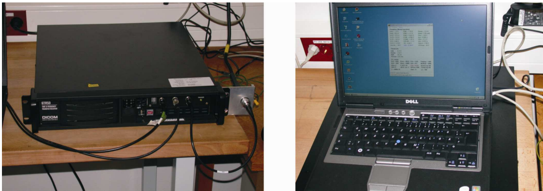
Figure 3.3.: GPS-receiver GTR50 and notebook: The left photo shows the GTR50. The notebook is placed on top receiver on the right photo.
