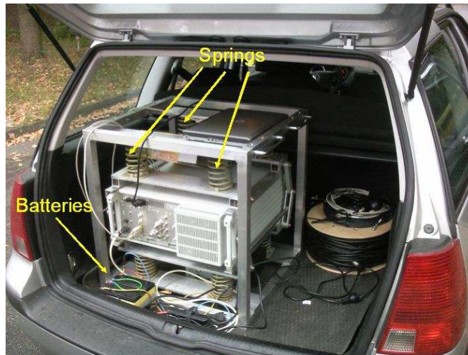
Figure 3.5.: The transportable maser inside the luggage space of a car.
