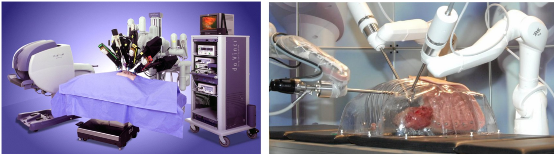
Figure 2.10: Examples of surgical robots: daVinci Surgical System, Intuitive Surgical (left); MIROSurge System, German Aerospace Center, Institute of Robotics and Mechatronics (right)
