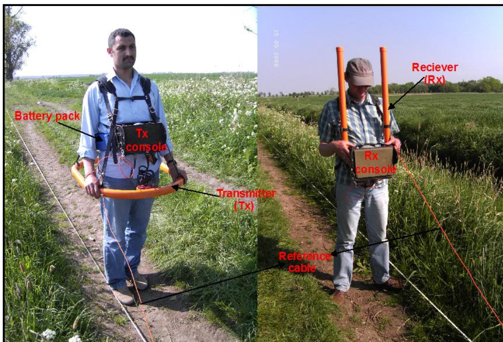
ig. 4.3: MaxMinI+10 EM instrument for FDEM measurements.
