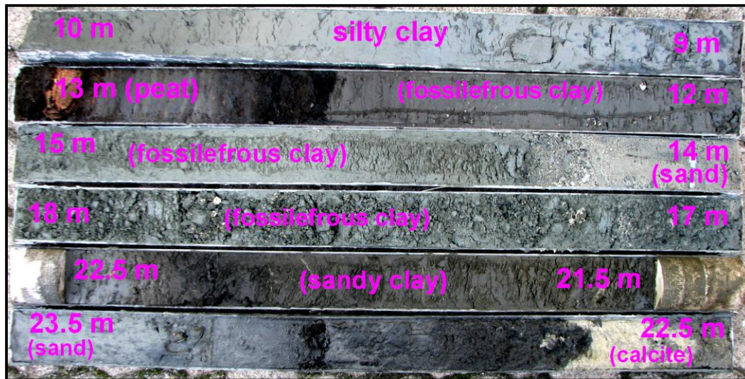
Fig. 5.48: Representative core samples from Eemian clay layer adjacent to the DS33 borehole location.
