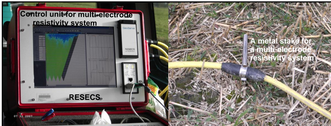
Fig. 4.2: RESECS multi-channel (8-channels) resistivitymeter for DC resistivity measurements.
