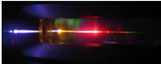
Figure 6.3: Picture showing the spectrally dispersed and focused octave-spanning spectrum in the Fourier-plane at the pulse shaper display. The blue-white left part of the line focus arises from artifacts due to capturing the infrared part of the spectrum.
