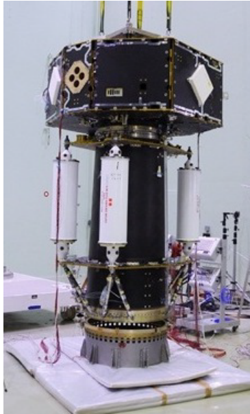
Figure 1.6: The LISA Pathfinder spacecraft composite. Science module on top of the propulsion module. Dummy tanks are attached to the propulsion module. The photograph has been taken during shock tests at ESTEC, The Netherlands, in October 2008. Source: [10]
