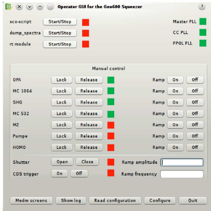
Figure 5.7.: Screenshot of the operator GUI for controlling the GEO 600 squeezed light source.
