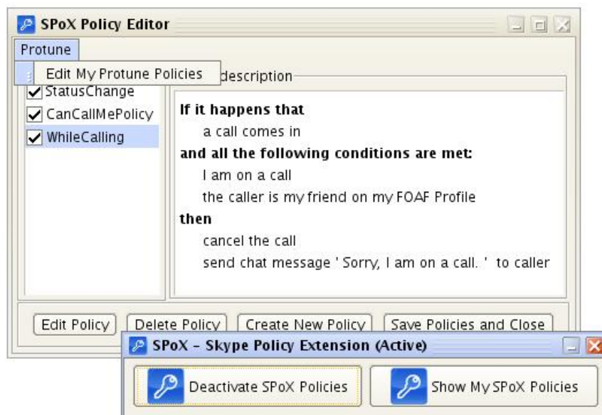
Figure 4.3: The control panel (bottom) and the policy panel with an overview of the current SPOX policies (top).
