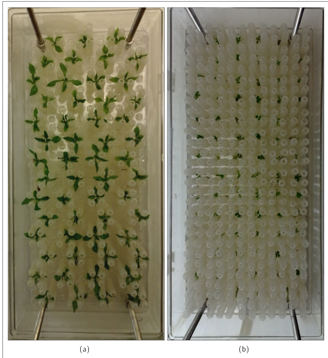
Fig. 4.2: PA-TIS carrier layout for two different cultures: a) 55 Malus shoots, b) 80 Kalmia shoots.
