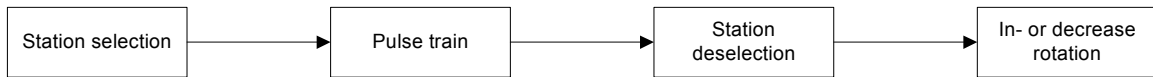
Fig. 8: Software sequence to individually change the stirring rates of the Tristation's agitation units.
