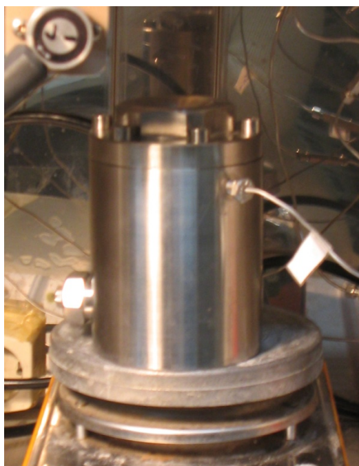
Fig. 4.2. High pressure reactor for scCO 2
