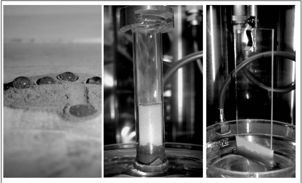
Fig. 28 Evaluation of wettability for a DCDMS-treated sample of silt. A: Water Drop Penetration Time. B: Capillary Rise Method. C: Wilhelmy Plate Method.
