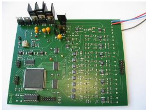
Figure 22: Photograph of dedicated temperature readout system.
