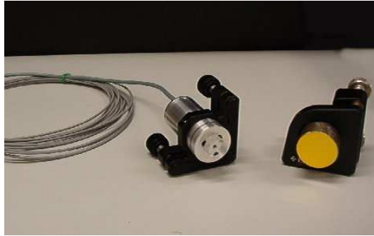
Figure 106: Comparison between PZT actuated mirrors (left) and static test mirrors (right).
