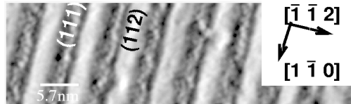
Abbildung 4.1: Si(557) imaged with STM. Periodic arrangement of alternating (111) terraces and (112) facets as suggested by Kirakosian et al. [12]. The size of one unit is 5.7 nm i.e. 17 atomic units.
