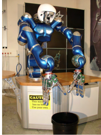
Figure 3.1: The DLR humanoid robot JUSTIN . The robot has 43 DoF. It is used for performing two-handed manipulation, object recognition, and grasp planning. A multisensory head as described in Chap. 7 is used for environment acquisition.
