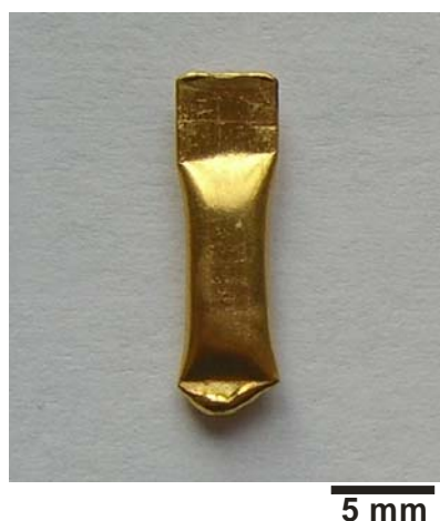
Figure A3.5. Photograph of an Au capsule used for isotope exchange experiments.
