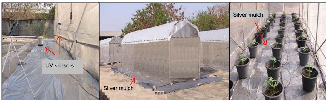
Figure 26. Experimental setup: Position of UV sensors (left), greenhouse and mulch arrangement from outside (middle), and inside (right).
