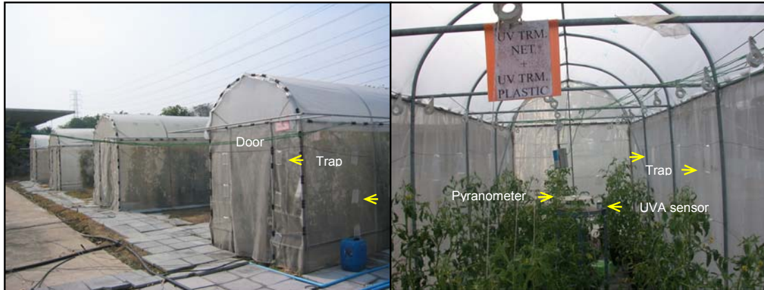
Figure 7. Greenhouse structure and experimental set up viewed from outside (left) and inside (right).
