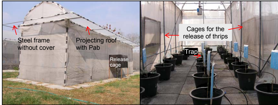
Figure 18. Experimental greenhouse design viewed from outside (left) and inside (right).
