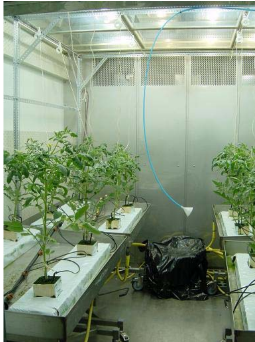
Figure 2: Construction of the climate chambers used and distribution of the tomato plants of the varieties FM TT260 and Pannovy on the transplanting day. Four plants per mat and eight plants per table (completely randomized) were grown on rock wool, fertigation was done automatically.
