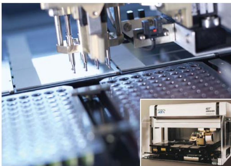
Figure (4.26): The Affymetrix 427 arrayer applies the ring and pin spot deposition technology whereby it is able to spot 42 slides at one time, with capacity up to 5000 spot per slides. The oligonucleotides are in 96 well microplates. The ring captures aliquots from the well and the pins deposit a fraction of fluid directly onto a slide surface (biochip).
