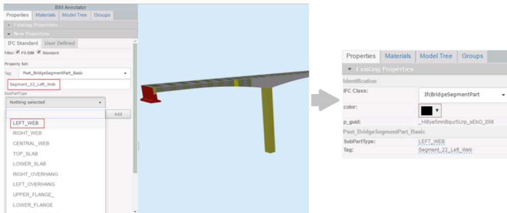
Fig. 14: Change the class and add new properties of a bridge segment part element
