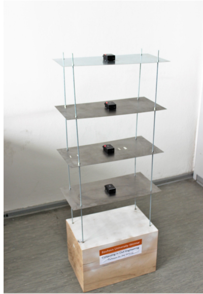
Fig. 1: Laboratory test structure instrumented with wireless SHM system.
