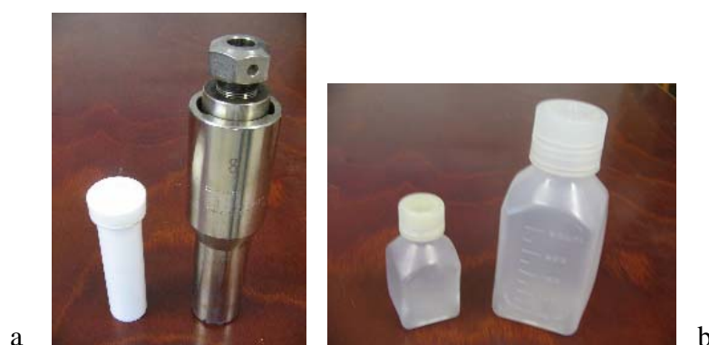
Fig. 4. Containers used in the syntheses. a) Teflon liner with the steel autoclave b) Polypropylene bottles (PP), 60 and 250 ml.
