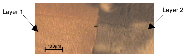
Figure 64: Test specimen used for the “concentration-distance” analysis (layer 2 contains DOP)
