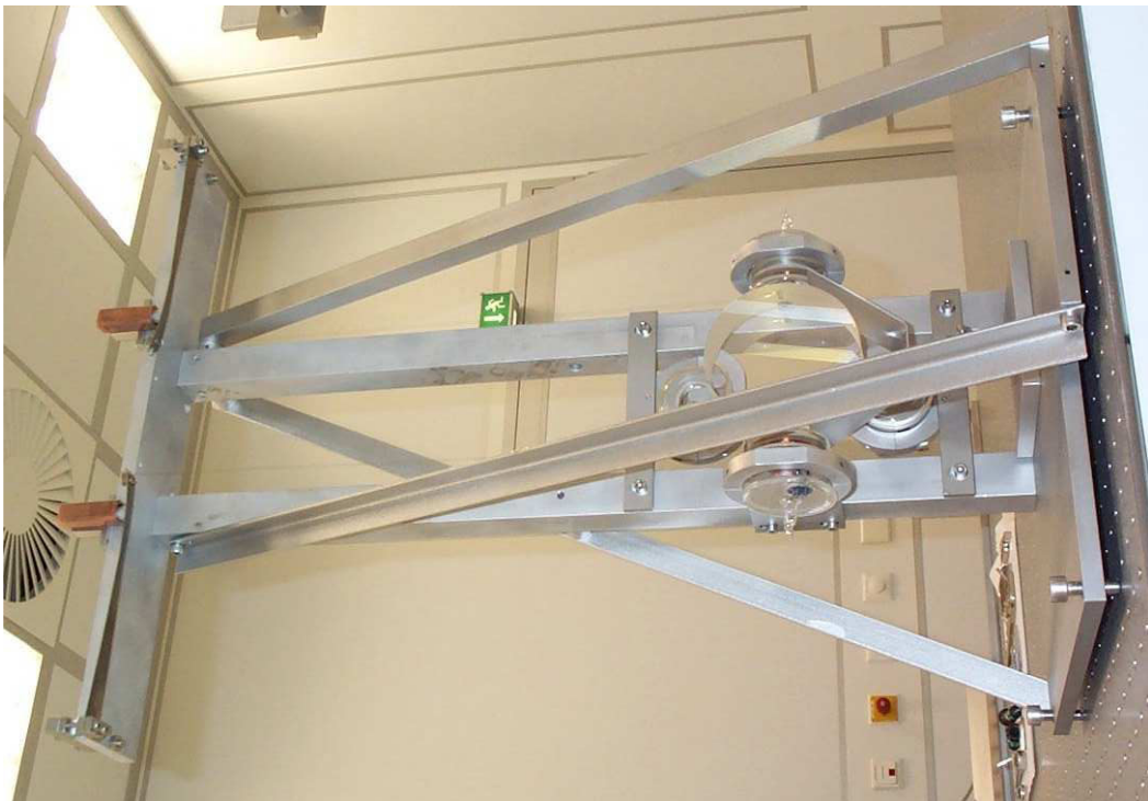
Figure A.2.: Suspension of BDO2. For BDO2 a stand alone Suspension is used which is clamped onto the bottom plate of TCOa.
