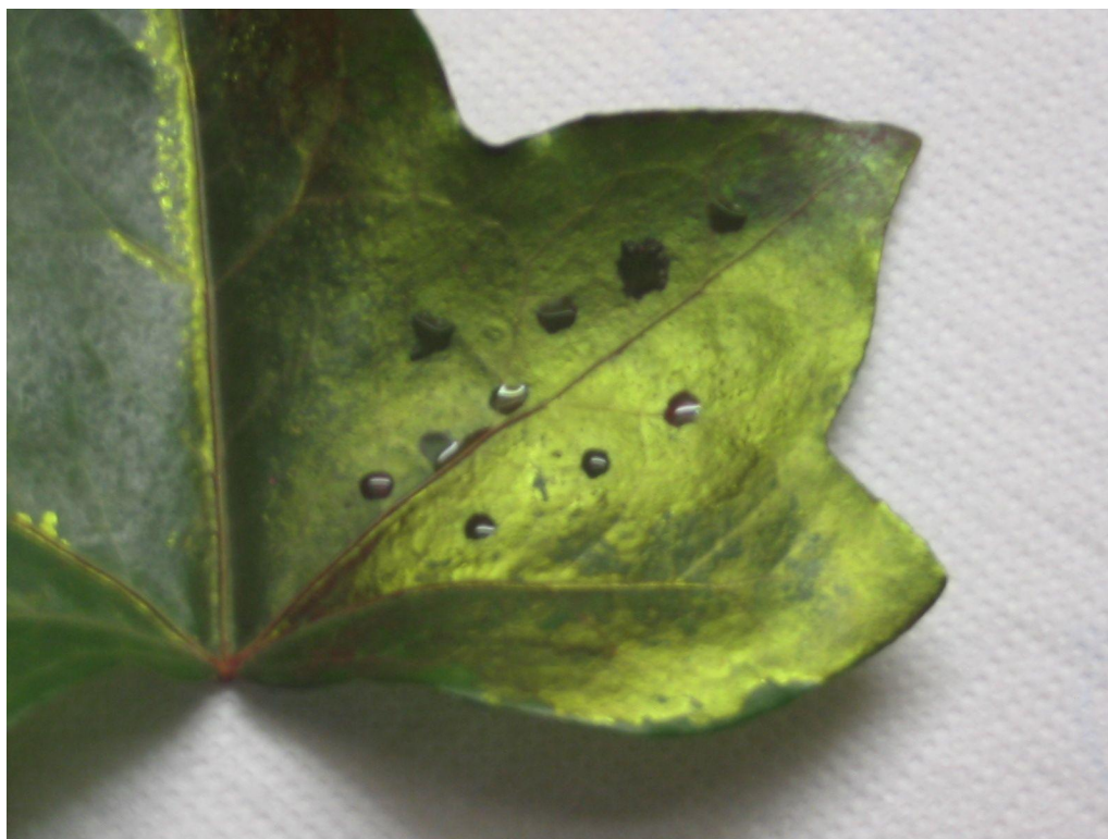
Figure 4.29: Fluorescence image of an ivy leaf ( Hedera helix ) recorded by a digital camera. The right half of the leaf was pretreated with a Rhodamine 6G layer, the left side was left untreated. On both sides droplets containing the sample pesticides were applied (not visible on the left side). Irradiation was done using an UV-C lamp and the fluorescence of the dye dissolved in the droplets can be observed on the right side while on the left side (not pretreated with Rhodamine 6G ) there is no notable emission.
