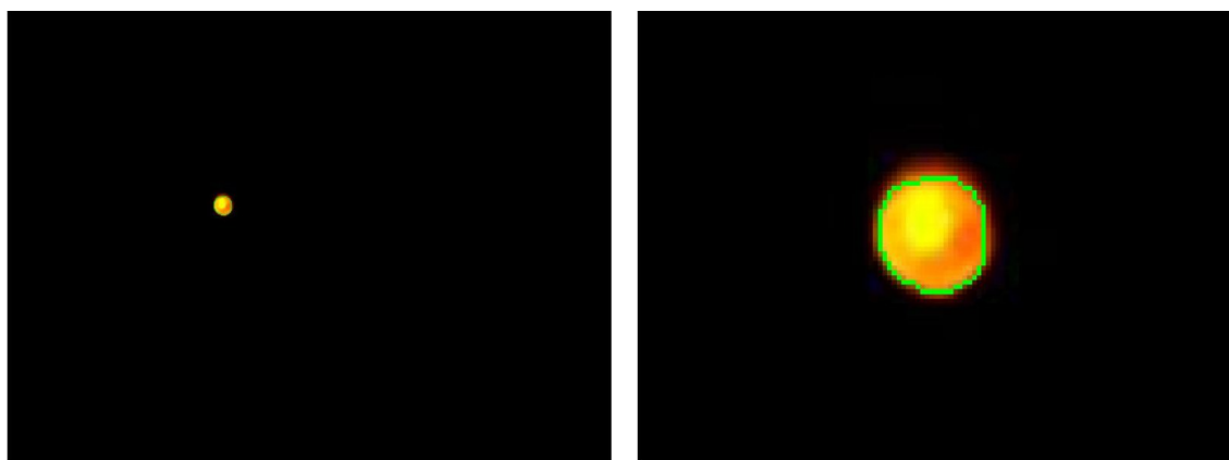
(a) The original color picture is shown. As overlay the detected edge is added outlining the plasma event.
