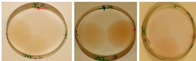
Figure 7.27: Samples number 2, 3, and 4 two weeks after the radiation tests. No spontaneous bleaching of the glass was observed.
