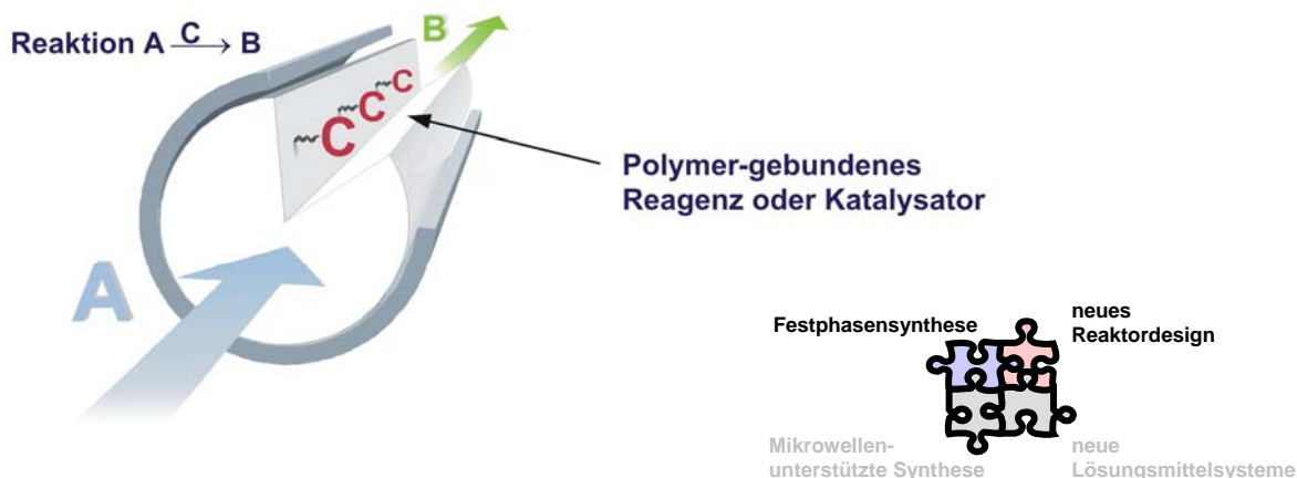
Abbildung 1.2: PASSflow -Reaktor ( Automated Polymer Assisted Solution Phase Synthesis by flowing through Monolithic Microreactors ).
