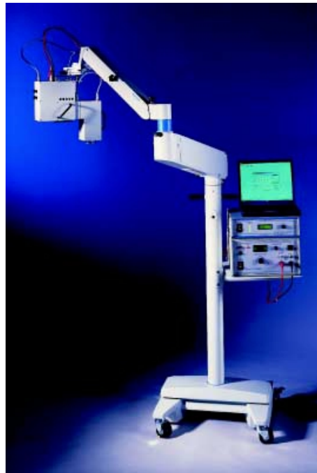
Figure 6.1: Solar simulator by M.U.T. as used in the experiments [49].
