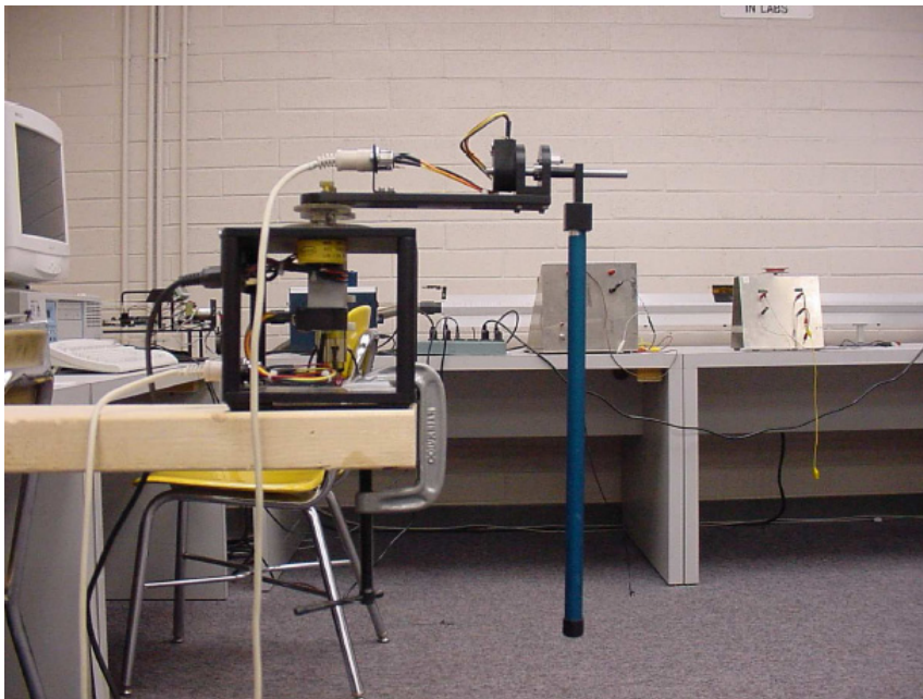
Figure 1.6 Laboratory setup for Furuta pendulum [Wan04]
