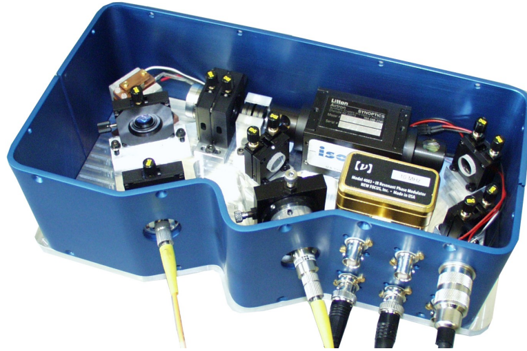
Figure 3.3.: LISA laser demonstrator with open top cover.
