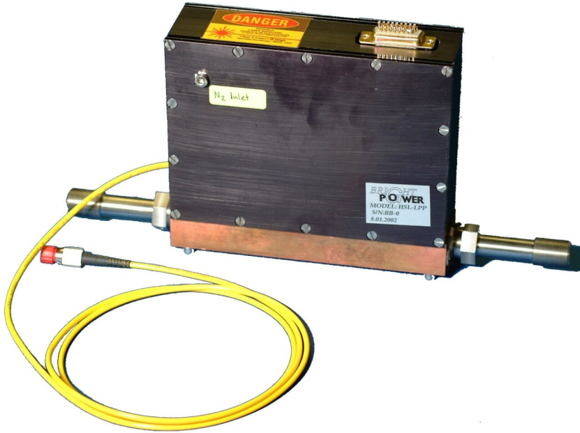
Figure 3.4.: Pump module for the LISA laser demonstrator.
