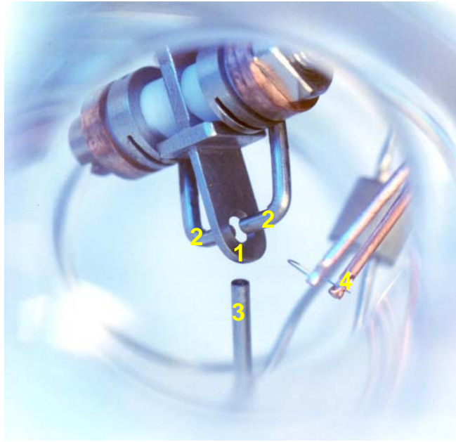
Figure 4.2: Picture of one of the traps used in the experiments. 1: ring electrode ( \text{\O}1.4 mm), 2: endcap electrode, 3: ytterbium oven, 4: electron source.
