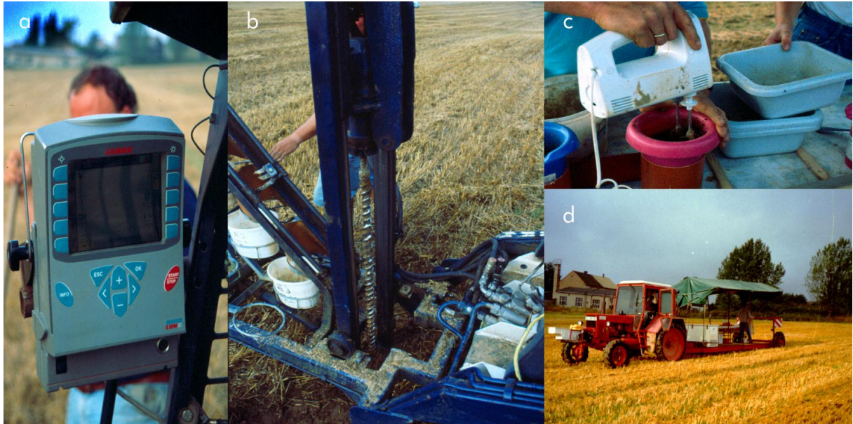
Figure 7. Equipment used for field campaigns. ACT-board computer for positioning (a), the mechanical auger (b), the mixing of soil samples (c) and the processing bench (d). Notice the large white freezer in d, which was used to cool the samples immediately after sampling and mixing. Images: Wendroth, Garlinski.
