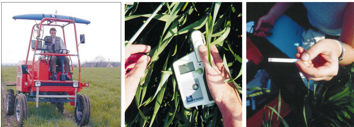
Figure 9. The HydroN-Sensor during a recording run in 2000, mounted on top of a lightweight vehicle (Left). Manual measurements of leaf chlorophyll content using the HydroN-tester (middle) and of the plant-nitrogen content using a Merck Nitrate test set (right). Images: Reuter, Wendroth.
