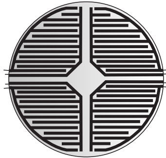
Figure 3.25: The electrostatic actuator used for the fast feedback at the mirror itself. The electrostatic actuator has eight comb-like interleaving patterns coated onto its front side. These patterns form four capacitors which can independently be charged with high voltage.
