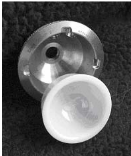
Fig. 1.3 Photograph of the acetabular components of a contemporary total hip replacement. The shell is usually made out of metal, and the liner may be ceramic, metal, or ultra-high-molecular weight polyethylene, from [6].
