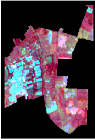
Fig. 6-6a, 1995, Landsat image before histogram matching
