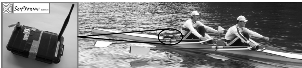
Figure 1. The training and measurement system Sofirow .
