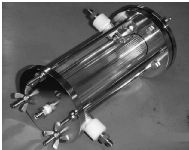
Figure 2.17. A photo of optical fiber photoreactor 72 . Reprinted from Ref 72 Copyright (2005), with permission from Elsevier
