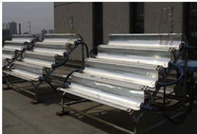
Figure 2.6. Direct solar photocatalytic hydrogen production reactor 45 . Reprinted from Ref 45 Copyright (2010), with permission from Elsevier
