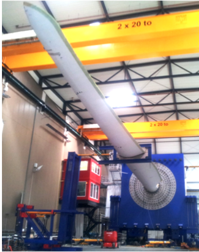
Figure 5.18: Test setup for fatigue test with load frame attached 17.5 m from blade root. Loading structure on the left.
