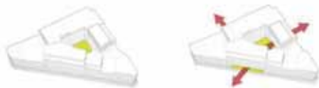
Figure 4: Building with an open space in its centre and passages for air circulation (Source: DRAKONTAEIDIS and PISIMISIS, 2017)
