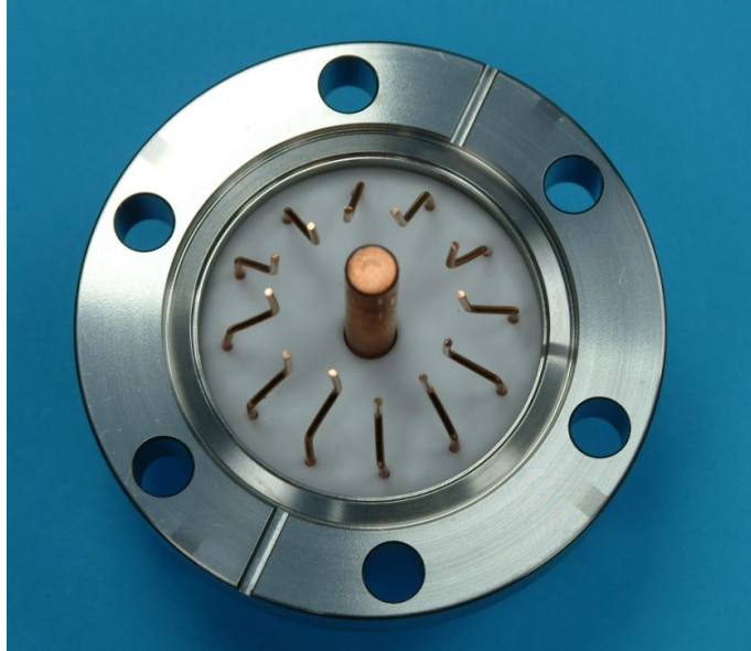
Figure 3.11. Custom-made vacuum feedthrough used in the trap setup of Figure 3.9. The central 6-mm conductor is the RF feedthrough; the surrounding pins are for the DC voltages and dispenser current. The insulator material (white) is alumina ceramic.
