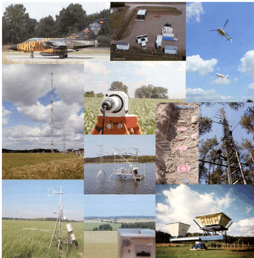
FIG. 4. Instrumentation during the LITFASS 2003 experiment (top left, left to right) Tornado aircraft, lidar and wind profiler Radio Acoustic Sounding System (RASS) at the central site (GM), helicopter with Helipod; (second row, left to right) GM with 99-m tower, and laser scintillometer over a maize field; (third row, left to right) micrometeorological station at a lake, soil sensors, forest tower; (bottom row, left to right) micrometeorological station over barley, large-aperture scintillometer path, boundary layer wind profiler at MOL.
