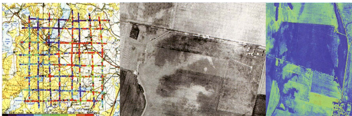
FIG. 5. (center) Infrared image of the area around the central site taken from a Tornado RECCE aircraft of the German Air Force and surface temperatures from the (left) Helipod, which were used to calibrate the infrared images and the calibrated infrared surface temperature from (right) the combination of Tornado and Helipod measurements. The reverse “L”-shaped central experimental site GM of roughly 300 m × 200 m size can be identified in the center picture and in the lower left quadrant of the right-hand picture. Temperatures in the left-hand picture range from 20° (blue) to 55°C (red).
