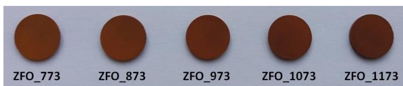
Fig. A9. Photograph of the ZFO samples with different degrees of inversion ( x = 0.074 \pm 0.011 , 0.104 \pm 0.013 , 0.134 \pm 0.008 , 0.159 \pm 0.010 , and 0.203 \pm 0.017 for ZFO_773, ZFO_873, ZFO_973, ZFO_1073, and ZFO_1173, respectively). As the degree of inversion increases, the brownish orange color of the samples becomes gradually darker.
