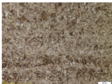
WEZ 2 Fine-grained martensite, HV1-500-520.
