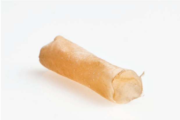
Figure 4: Electrospun tubular protein based scaffold treated with glutaraldehyde vapour (diameter: 6 mm, length: 20 mm). ©: Daniel Kühnhold, 2016.
