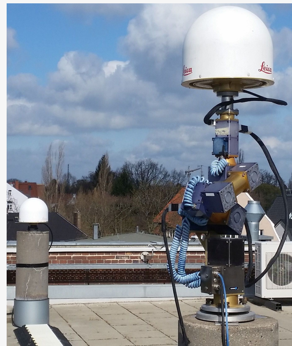
Figure 1: IfE robot for absolute antenna calibration. In the background the reference station (MSD8) can be seen.
