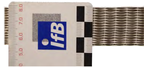
FIGURE 2. Unidirectional carbon fibre band
