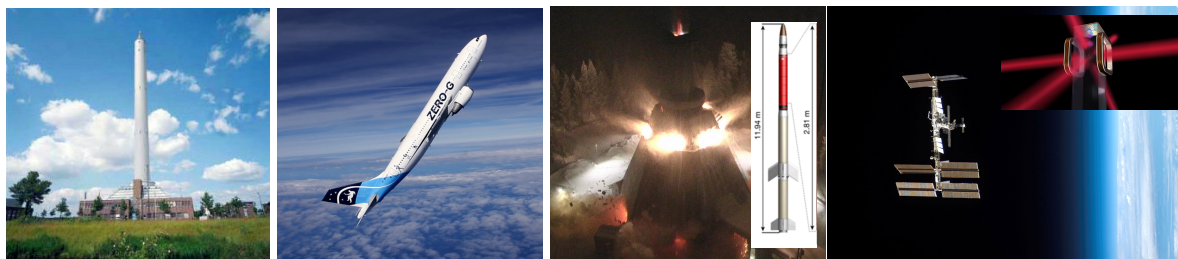
Figure 1.3: Different micro-gravity environments. From left to right, the Bremen drop tower experiment, the zero-g-Airbus A310, the launch of the Maius-1 sounding rocket, the International space station (ISS) and the CAL experiment. The different pictures were respectively taken from [174–180]
