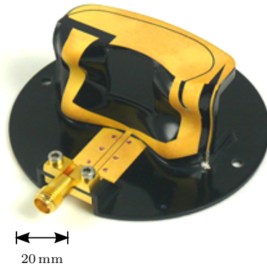
Figure 3.2 Realized prototype of a surface modulated broadband monopole with shorted top-load and additional slot.
